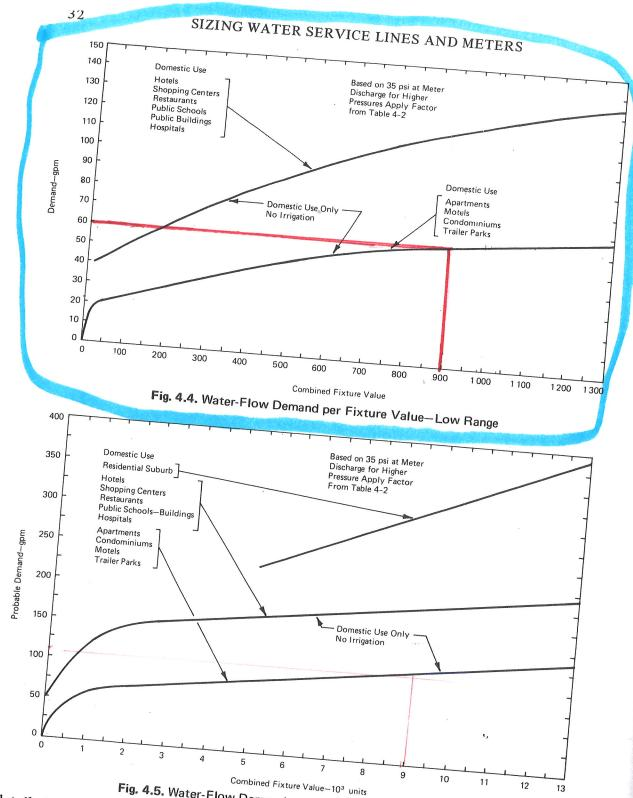
Fig. 4.5. Water-Flow Demand per Fixture Value—High Range detailed lists of fixtures before estimates can be prepared. If the structure is in the planning stage, the mechanical engineer or architect is the best source of information, and, if construction is underway, the plumbing contractor or the building permits section of the city will have the information. Field trips by the estimator are often necessary to assist the customer as well as to properly assess the project when
